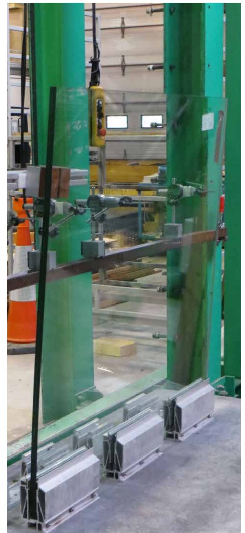
Figure 1 Overview of balustrade testing for thicker configurations (1010.x and 1212.x)
