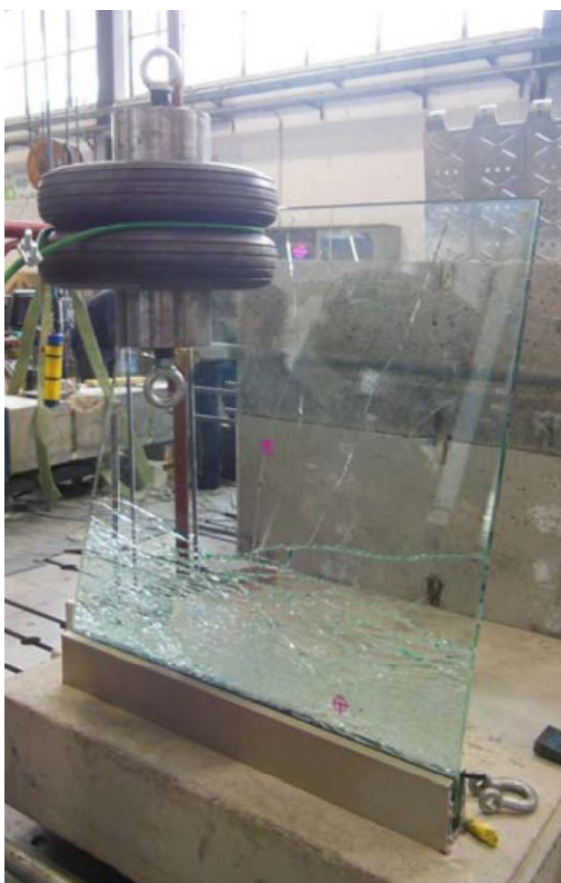
Picture 3 & 4: Post breakage behaviour annealed laminated stiff PVB .
